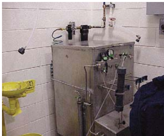
Figure 2. Test apparatus for NSF/ANSI 61 municipal exposure of activated carbon
