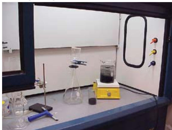
Figure 2. Test apparatus for NSF/ANSI 61 municipal exposure of activated carbon
