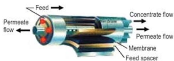
Figure 1. Spiral-wound membrane element
